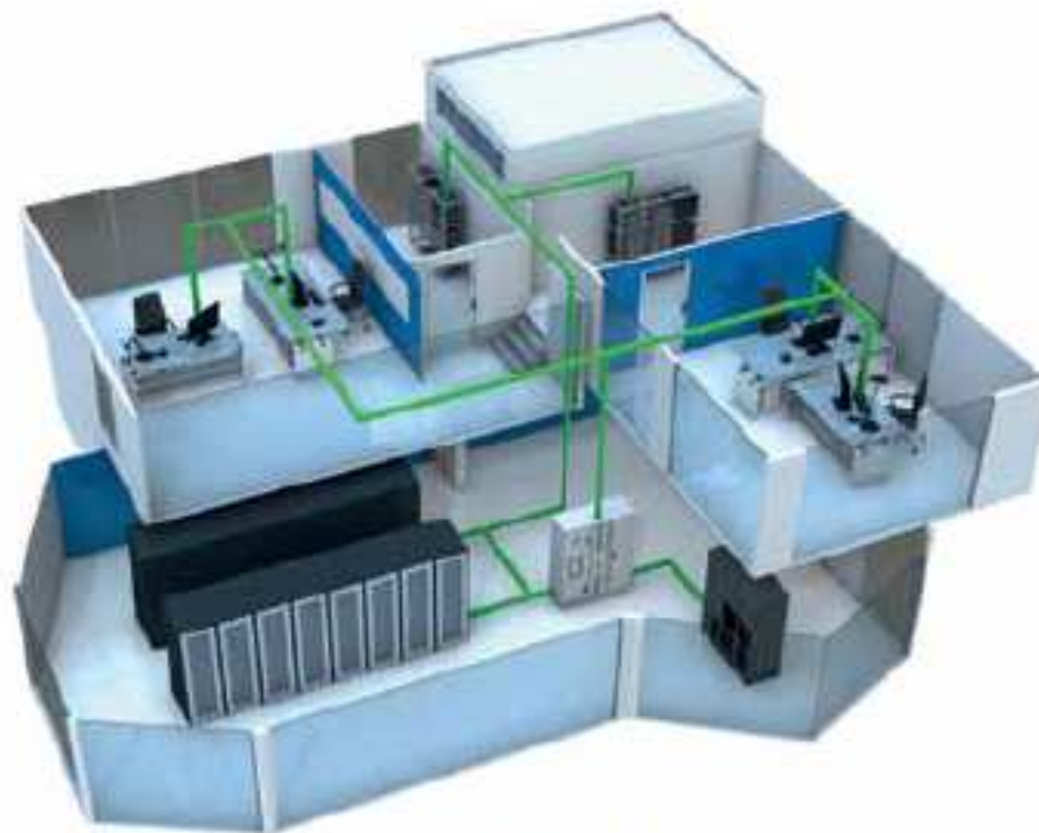
Centralised UPS solution.
